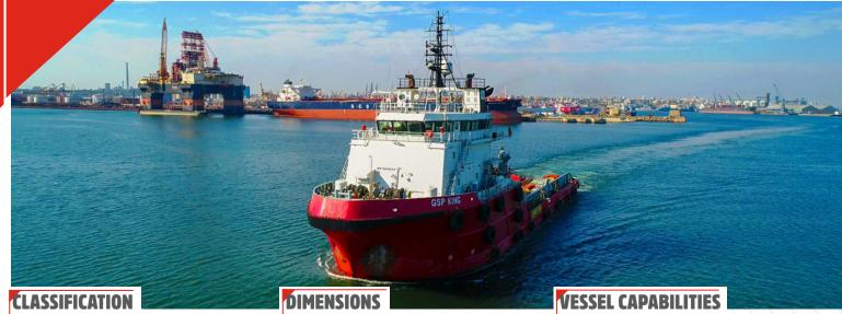
**★A1**, Towing Vessel, Fire Fighting Vessel Class 1, Offshore Support Vessel, ©, ★ AMS, ★ DPS-2
